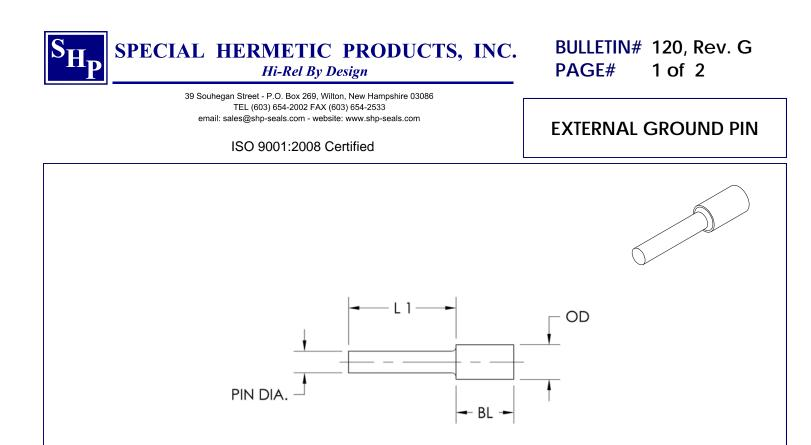
This ground pin is designed for ease of solderability in a variety of housing materials as well as for high solder joint reliability in severe thermal cyclic environments. Its enlarged base and application geometry facilitate plating in the blind bore, thereby ensuring a sound solder joint.
